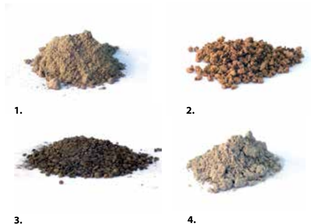
1. Diatomaceous earth / 2. Cork / 3. Clay / 4. Natural hydraulic lime
