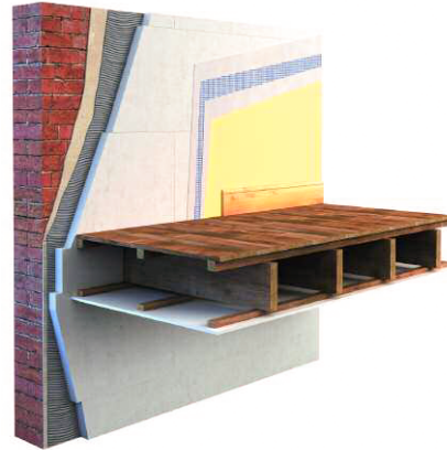
Insulated ceiling joist (wall continuously insulated)
