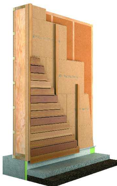
External EcoWall Construction
