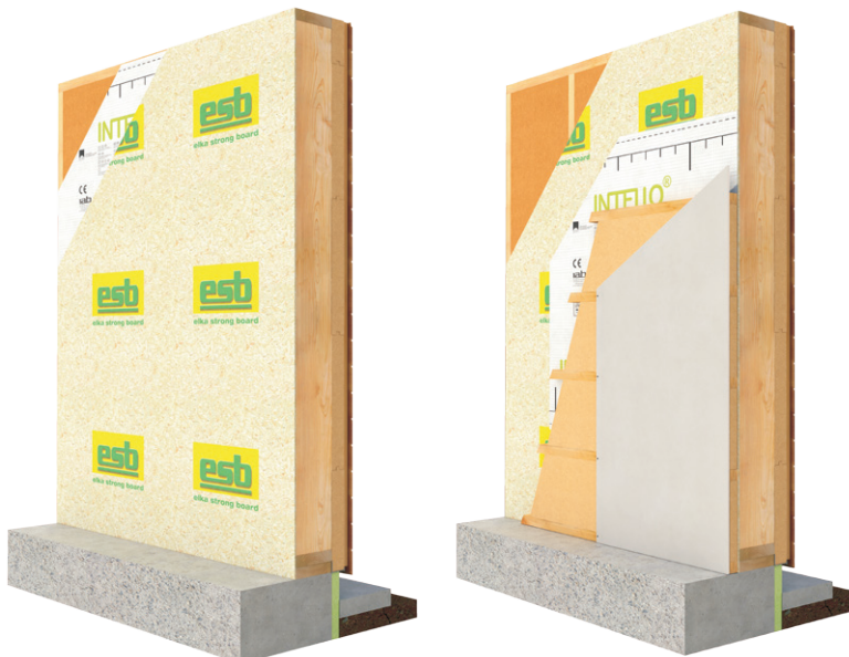
ESB boards can be applied internally & painted directly or dry-lined
