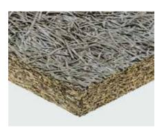
Thermal and acoustic insulation board, consisting of mineralized fir wood wool bound with grey Portland cement. Wood wool is 3 mm wide.
