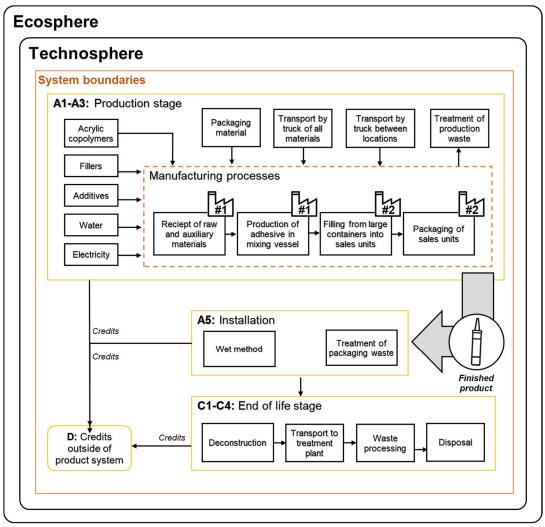
Each processing step within the system boundaries is marked with an icon and number (#1, #2, etc.), indicating the specific production site where it occurs. The system boundaries cover the following modules:
