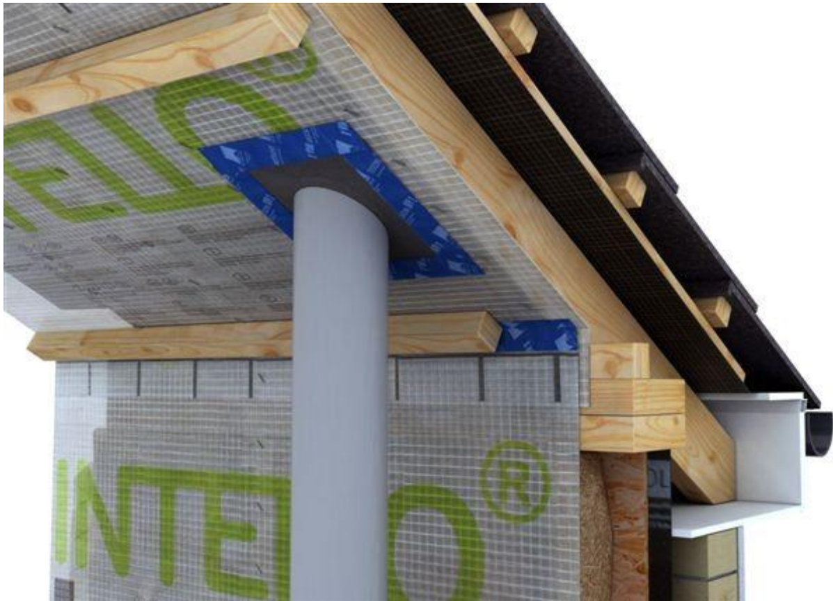
Figure 4: Roof detail with pipe grummet
